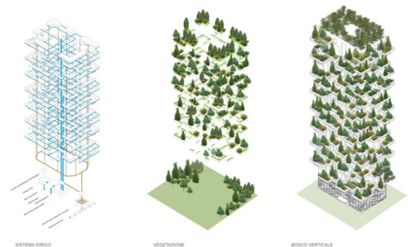
Figure 5. Bosco Verticale, Stefano Boeri & partners 2014. Detail of the construction system.
